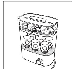
**Note:** When you fill the small basket, put screw rings on the bottom, place the teats and the bottle caps loosely on top of the screw rings.
